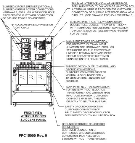
Figure 7 Electrical connection location for 47" (1194mm) cabinet—Rear view
